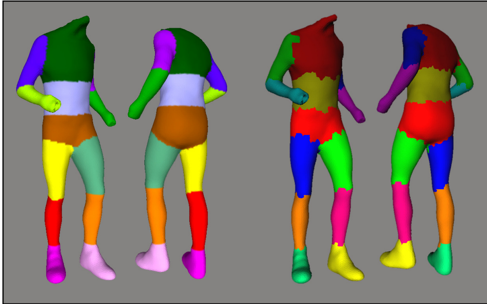
Figure 3. 18 Ground truth segmentations. Left: The initial ground truth segmentation. Right: The ground truth segmentation used for error calculation.
