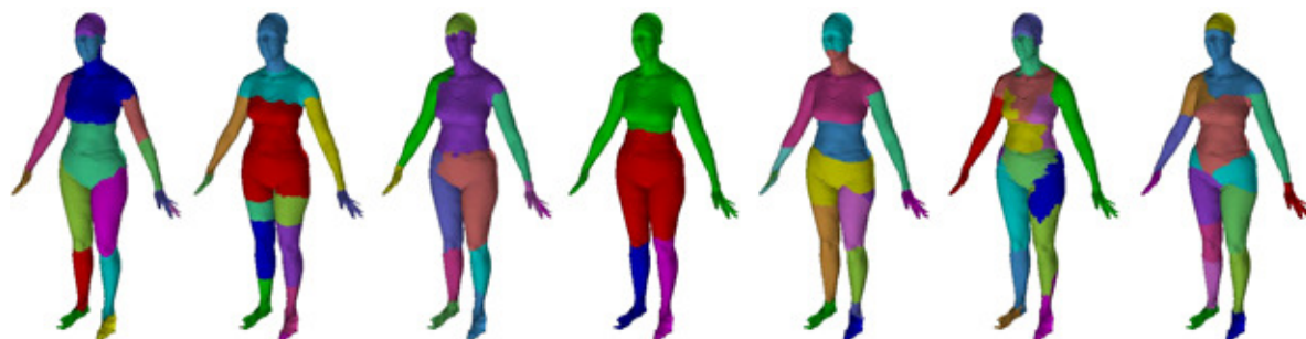
Figure 1. 1 Segmentation results for a static human model extracted from [3]. From left to right, Randomized Cuts [4], Shape Diameter Function [14], Normalized Cuts [4], Core Extraction [7], Random Walks [9], Fitting Primitives [1] and K-Means [15].
