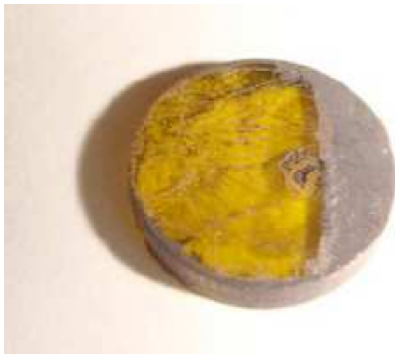
Figure A.1: ZnSe crystal after being etched in the \text{KMnO}_4 , \text{H}_2\text{SO}_4 and DI water solution.
