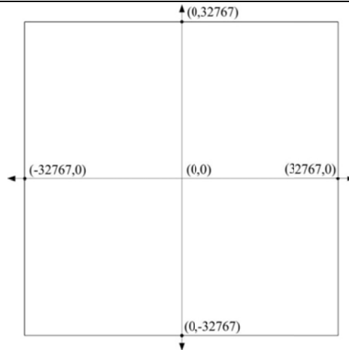
Figure 4.6 Scanning system field size and bit number relation
