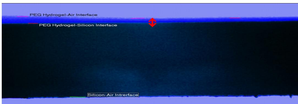
Figure 3.3 – Thickness measurement method of PEG hydrogel on the silicon surface via optical microscopy
