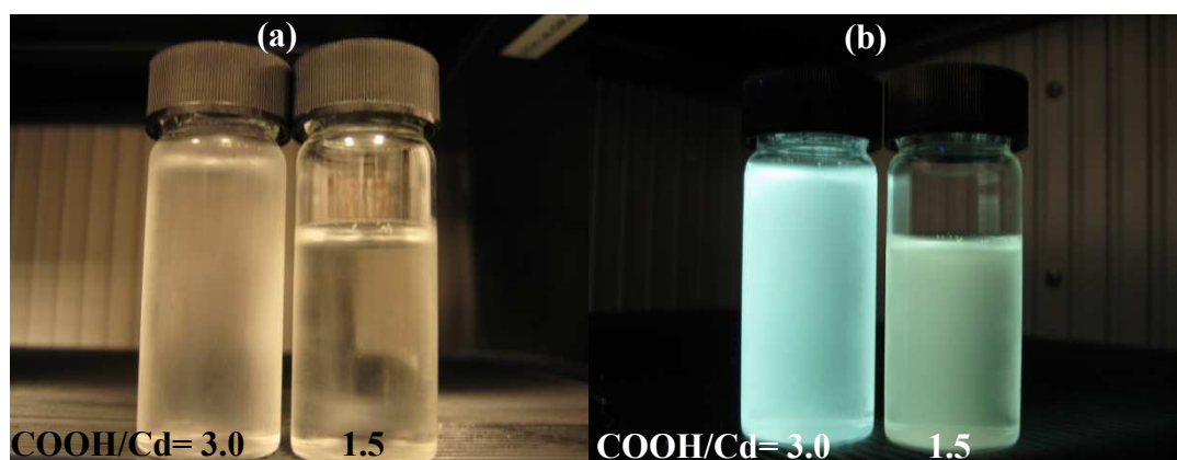
Figure 3.8 Pictures of the P(AAA)/Cysteine (60/40)-CdS nanoparticles under (a) daylight and (b) UV excitation ( \lambda_{\text{exc}} ) 366 nm.
