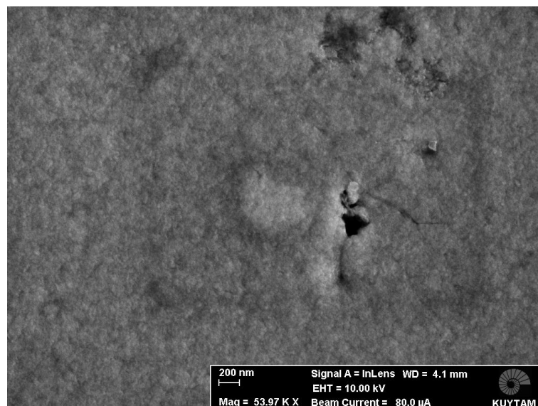
Figure 3.38: This microstructure of 500 nm thick nickel layer seems to have similar grain size with the other two samples
