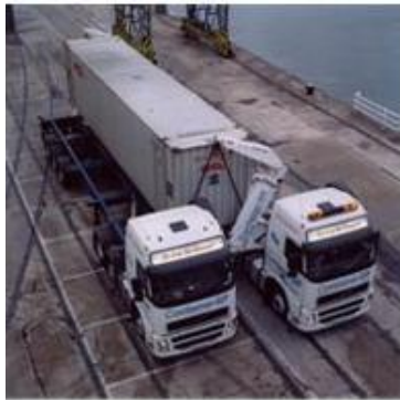
Figure 9: Loading of a container from truck to truck.
