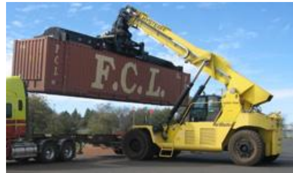
Figure 10: Truck loading by a top-lift type material handling equipment.
