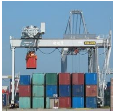
Figure 7: Yard crane (rail tired gantry crane).
