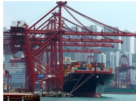
Figure 5: A berthed vessel and a quay crane assigned to that vessel.
