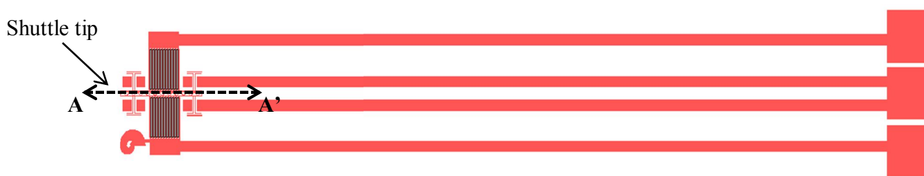
Figure 6.2: The force sensor design for mechanical characterization
