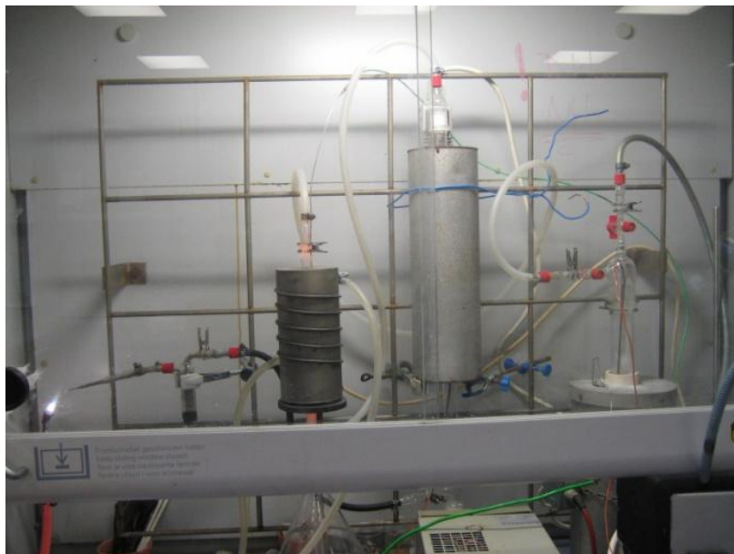
Figure 3.12 Third experimental setup with total yield of around 50 % of calculated boron amount
