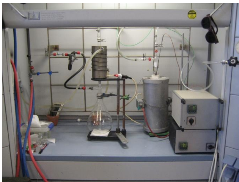
Figure 3.11 Second experimental setup with total yield of around 30 % of calculated boron amount
