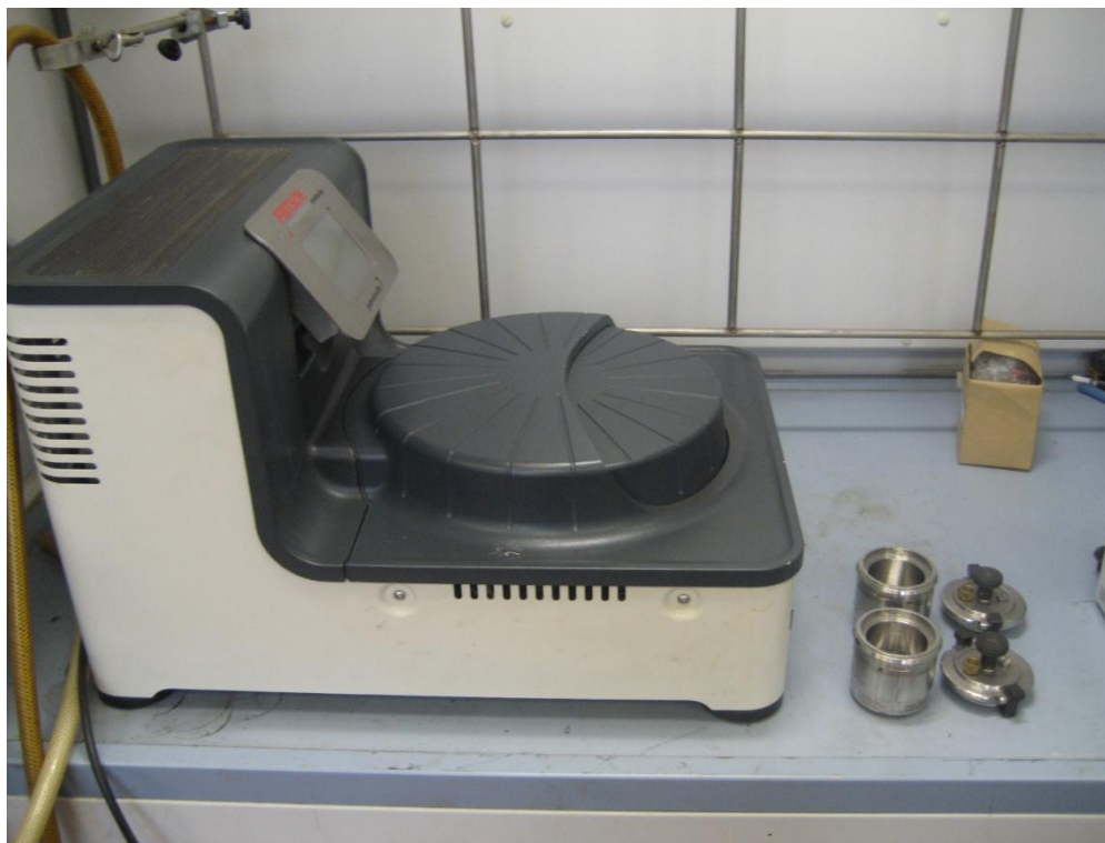
Figure 2.18 Fritsch Pulverisette Premium Line 7 planetary ball milling device with stainless steel grinding equipments.
