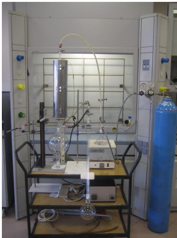
Figure 3.14 Final version of the experimental setup with total yield of around 85 % of calculated boron amount
