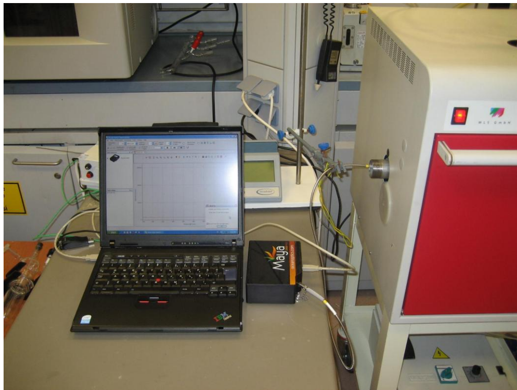
Figure 2.11 Emission spectrum measurement of hydrogen plasma
