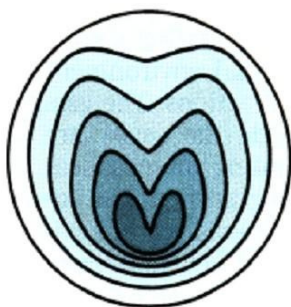
Figure 1-30. Scheme of the stages of a cavity implosion near a surface and the formation of the liquid jet [551].
