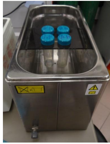
Figure App-4. Positioning dispersion vessels in ultrasonic-bath – side view.
