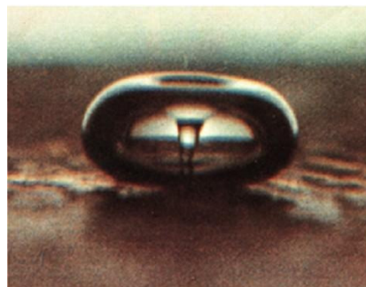
Figure 1-31. Photomicrograph of a liquid jet (size of the bubble is \sim 150 \mu\text{m} ) [551].
