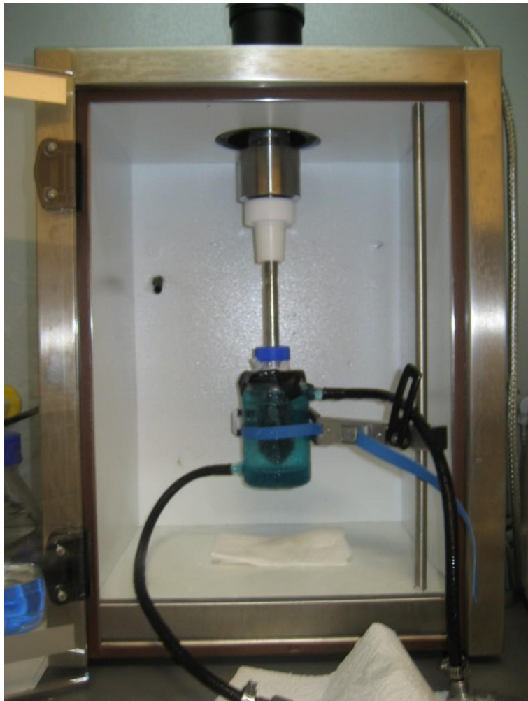
Figure App-5. Immersion of ultrasonic horn in dispersion vessel (Note that the vessel is located inside a cooling jacket and sample is dark which denotes dispersion of carbon nanotubes).
