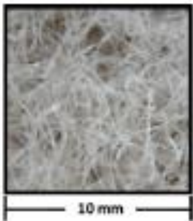
Metyx Meticore 250PP Polypropylene core 250 gram/m 2
