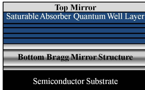
Figure 2.3.1 Schematic description for a semiconductor saturable absorber mirror (SESAM).
