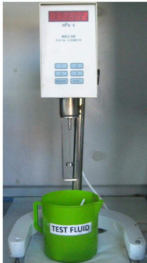
App C.11. NDJ-5S digital rotary viscometer
