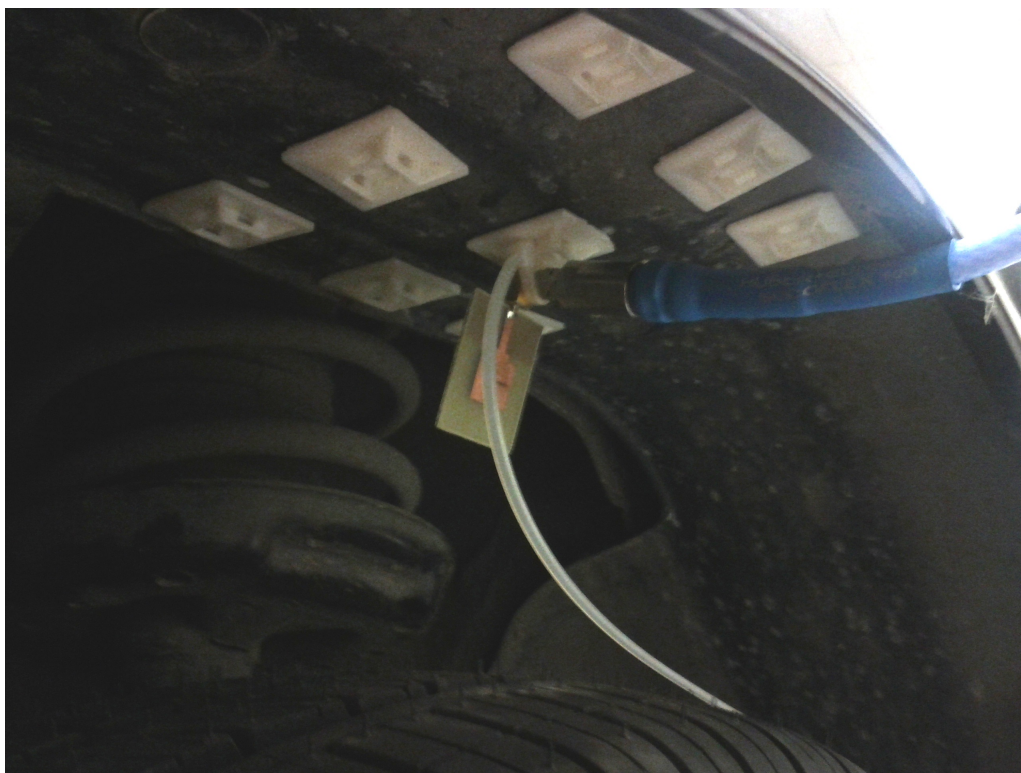
Figure 2.2: Sensor locations arranged in 3 \times 3 square grid for both transmitter and receiver
