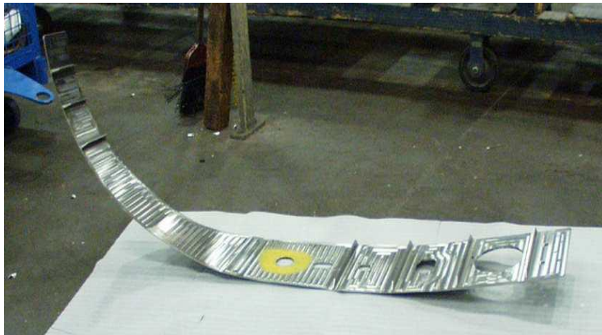
Figure 4: Distortion of a part due to residual stresses [Safran]
