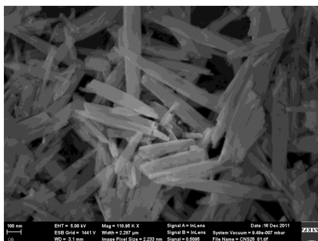
Figure 2.14 Effect of the absence of Yb 3+ on the shape of β-NaYF 4 microcrystals. Scale bars is 100nm. (Reaction conditions: Ln 3+ :Na + = 1:20, Ln 3+ :F - = 1:3, T=50°C, 3/3 sec pulse on/off, Amplitude= 50%, Dopant: Only Tm 3+ (2%))
