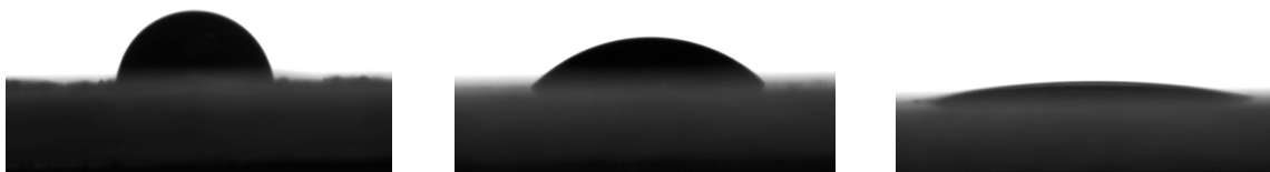
Figure 4.33 5 \mu l water droplet on the membrane which was templated from the emulsion of internal volume fraction 0.33, and particle concentration 0.7 % a) immediately after disposal of droplet (WCA = 80°) b) 1.5 seconds after (WCA = 25°) c) 2 seconds after disposal of drop (WCA = 13 °)
