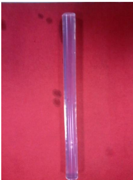
Figure 3.2.2: Cylindrical silica wet gel prepared in the laboratory (1.19 cm in diameter x 15.92cm in length)
