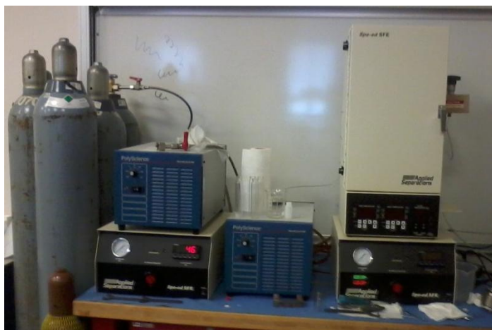
Figure 3.3.2: Drying Equipment of Applied Separations Speed SFE
