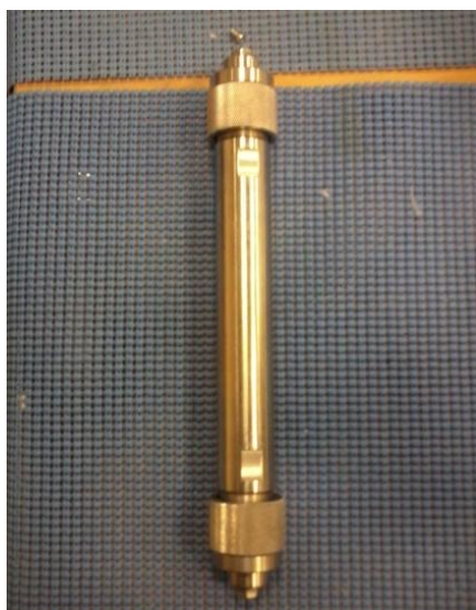
Figure 3.3.3: Extraction vessel (tubular reactor, length=15.94 cm, diameter=1.43 cm, volume=26 ml)
