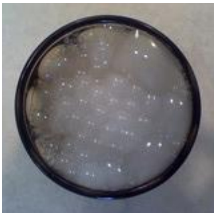
Figure 3.3.4: Dry ice bath prepared to maintain the outlet stream at low temperature
