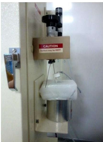
Figure 3.3.4: Dry ice bath prepared to maintain the outlet stream at low temperature
