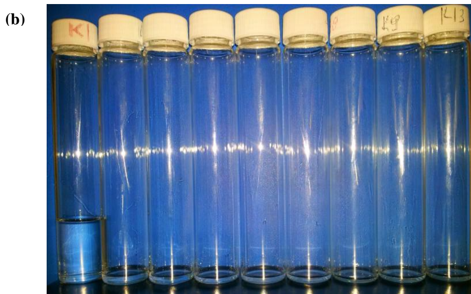
Figure 4.4.2.1: Ethanol extracted from the pores of the wet gel in the certain time intervals during the supercritical drying experiment in the laboratory.
