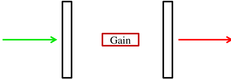
Figure 2.3: A sketch of a simple laser cavity
