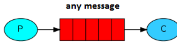
Figure 2.4 Simple operation of RabbitMQ. “P” represents “Producer”, “C” represents “Consumer”. Messages published by producers are sent to a queue. Messages are stored on the queue. Consumers wait to receive messages.
