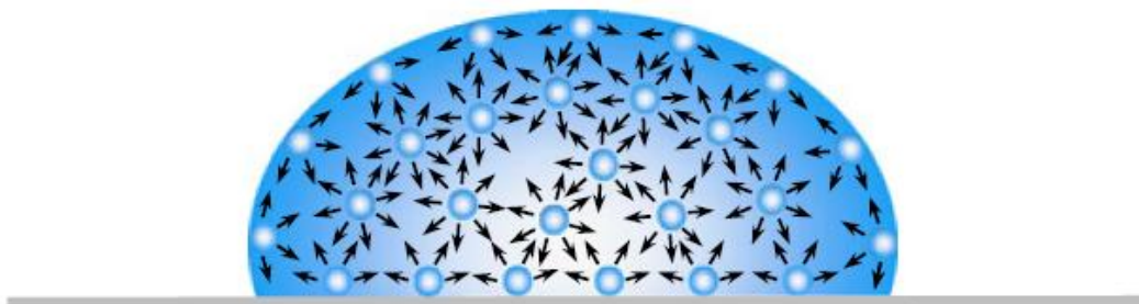
Figure 3. 9. Surface tension is caused by the unbalanced forces of liquid molecules at the surface
