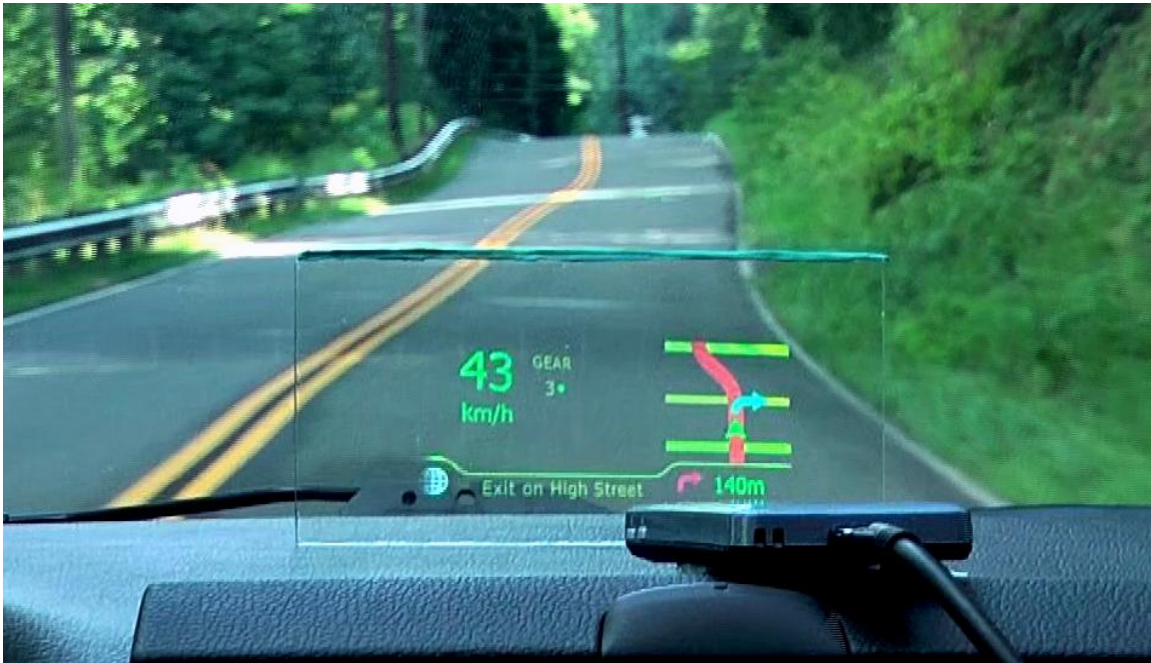
Figure 2.18: The demonstrator of the automotive direct projection HUD.
