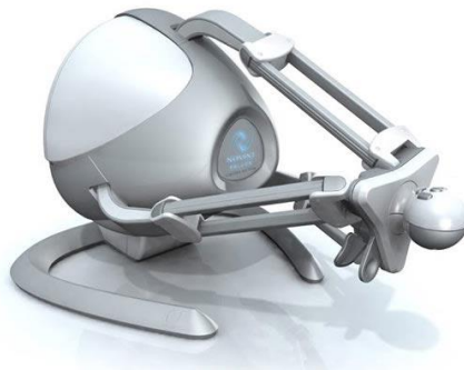
Figure 3.7 a desktop haptic robot Novint Falcon
