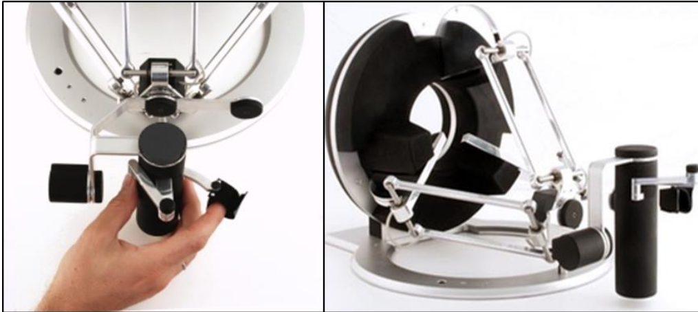
Figure 3.6 a 7-DOF haptic device ForceDimension omega 7
