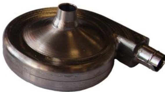
Figure 3.4 – Final Ti-6Al-4V prototype of previous study
