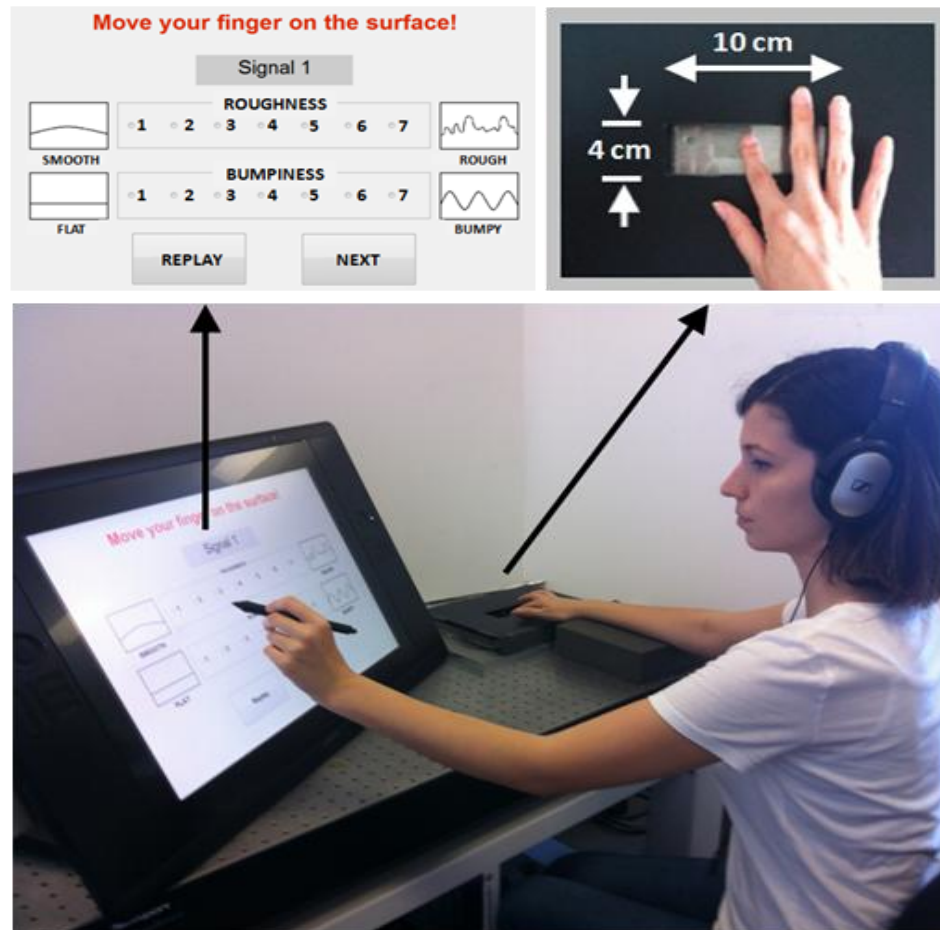
Figure 4.3: The experimental setup and the graphical interface used for the human experiments.
