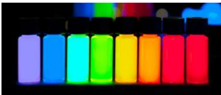
Figure 5.1.2: Band-gap tunable emission from colloidal quantum dots under ultra-violet excitation.
