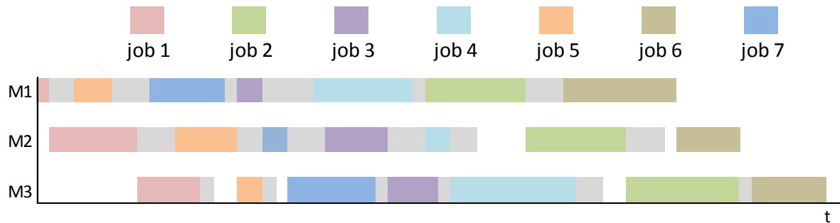
Figure 3.2 Gantt chart for the FS-SDST while minimizing the total production cost
