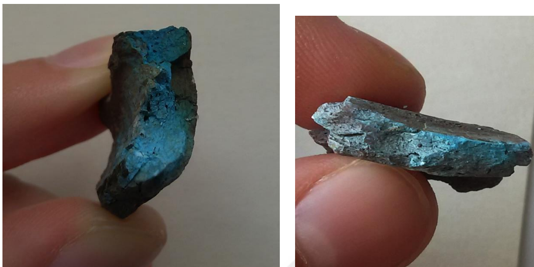
Figure 66 The same piece of archaeological sheep/goat bone sample part of the 3 rd batch that has been subject both to the solution and heat treatment. A) When heated at 600 °C for 26 hours. B) Same piece of bone heated for 18 hours more at 650 °C, totaling 44 hours.
