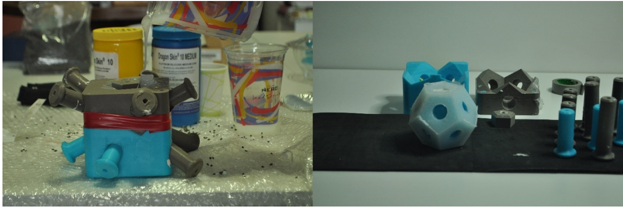
Figure 14: Molding process of the silicone cover of the Luck Stone
