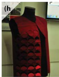
Reform Season comes forwards as a jacket that can be worn in different conditions such as indoor/outdoor, warm/cold weather since its pattern create holes for air circulations. They react to the outside temperature by creating different patterns via servo-motors and temperature sensors.
