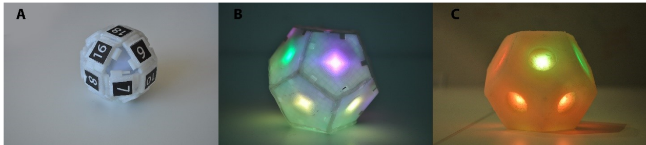
Figure 13: Evolution of the Luck Stone, (A) Luck Globe with Sphero, (B) Luck Stone without the silicone cover, (C) Luck Stone with the silicone cover
