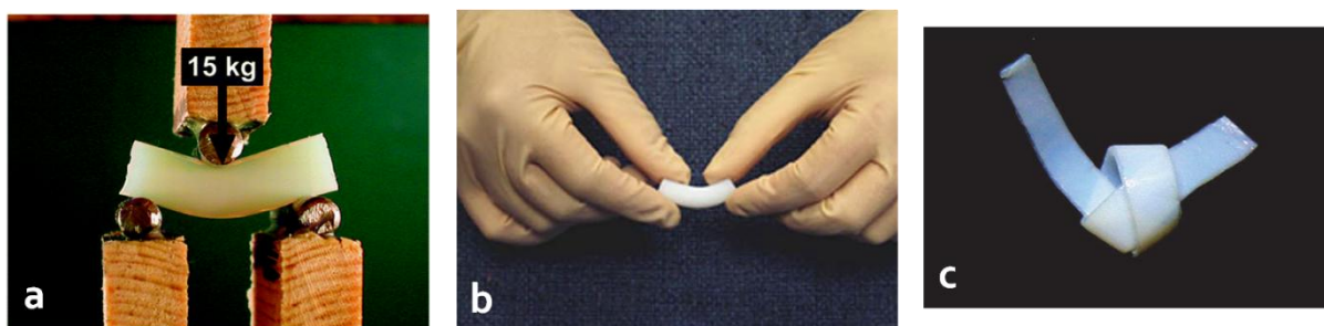
Figure 1 Composites of silica aerogels with a) poly(hexamethylene diisocyanate) [4] b) di-isocyanates [5] c) cellulose [6]
