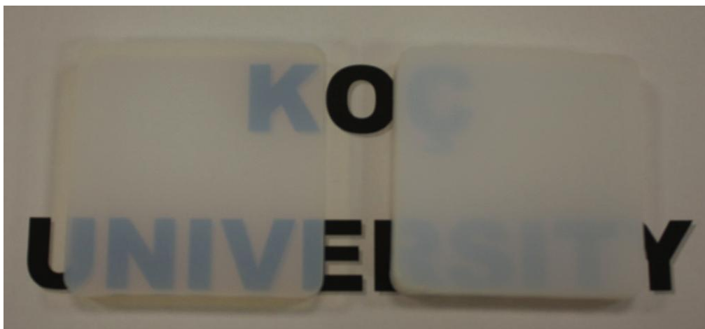
Figure 87 6.5 \times 6.5 \text{ cm}^2 silica aerogel samples with densities; 0.183 \text{ g/cm}^3 (left) and 0.272 \text{ g/cm}^3 (right).
