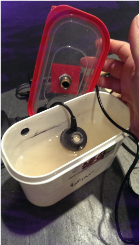
Figure 5: The inside of the scent machine, which held the piezoelectric motor, water, and drops of the scented oil.
