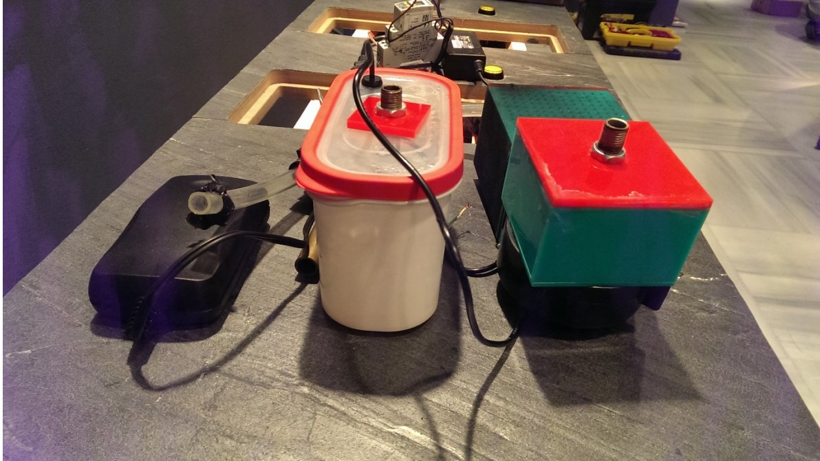
Figure 6: The scent machine. The power adaptor is on the left, the water and scent container in the middle, the charcoal filter and fan on the right, and the clock timer in the back.
