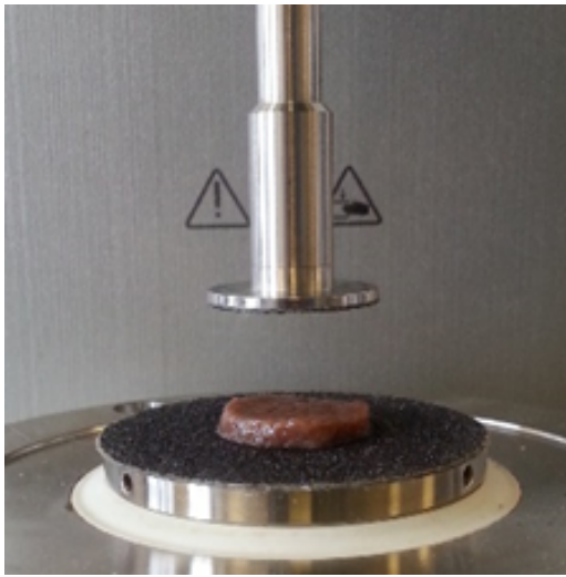
Figure 2.1: A liver tissue sample on the lower plate of the rheometer.
