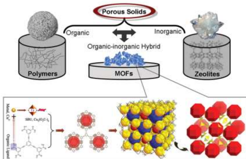
Figure 1.1 General classification of porous solids: polymers for porous organic solids; zeolites for porous inorganic solids and MOFs for porous hybrid solids.[3]
