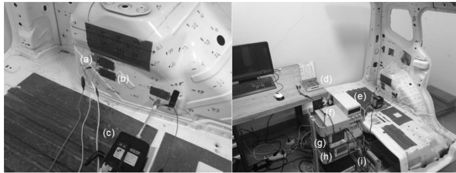
Figure 3. 4 Details of the experimental set-up a) PZT actuator b) PZT sensor c) Shaker d) Controller Unit e) DC Power Supply f) PZT amplifier g) Oscilloscope h) Signal Generator i) Signal Analyzer
