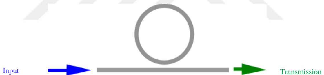
Figure 1.5: A channel-dropping filter realized with a ring resonator.
