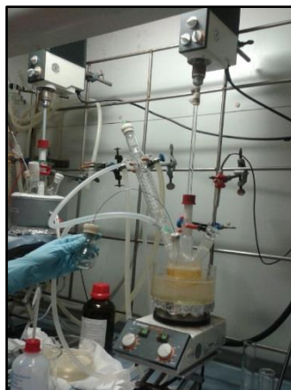
Figure 2. 1 Synthesis of PEI and 2MPA coated Ag 2 S NIRQDs.
