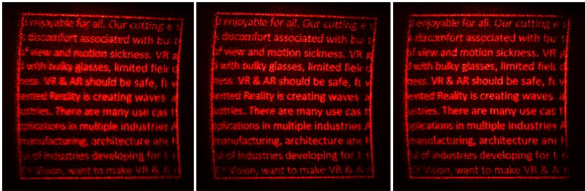
Figure 3.6. Effects of aberration and distortion correction. The original image (left) was corrected for aberrations to obtain the image at the center. Distortion correction was used to correct the corners of the image, resulting in the image to the right.
