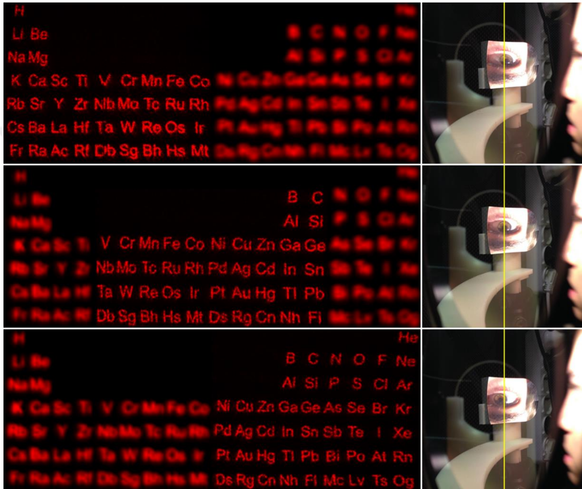
Figure 4.4. Experimental results of the eye-centric foveated holographic display. The periodic table is displayed by the SLM. As the eye rotates, a high-quality holographic view of different regions of the image is seen.
