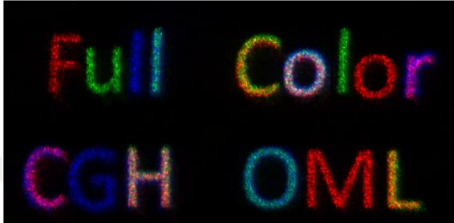
Figure 4.8. Holographic image with non-primary colors. The absence of refractive optical elements eliminates chromatic aberration, which greatly simplifies the generation of images with various color combinations.
