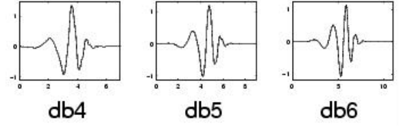
Şekil 2.19: Daubechies dalgacıkları [21] C_i = g_0 s_{2i} + g_1 s_{2i+1} + g_2 s_{2i+2} + g_3 s_{2i+3} C[i] = g_0 s[2i] + g_1 s[2i + 1] + g_2 s[2i + 2] + g_3 s[2i + 3]
