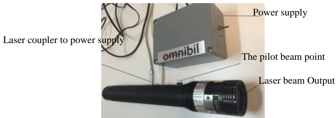
Figure 2.1 The 1940 Diode laser system. The Laser connector to the power supply, the power supply, the pilot beam point and the laser beam output are shown. The laser optical parameters are determined inside the laser
