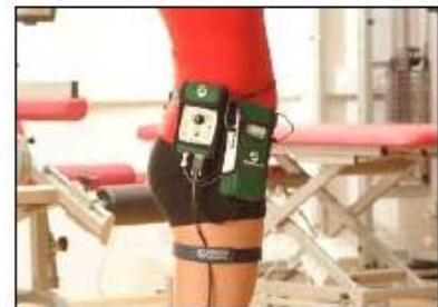
Depending on the need, the Multi-Mode FootSwitch System may be connected to the Telemyo G2 Transmitter "Digital In" or EMG ports.
