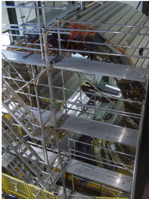
Figure 5.2. A photograph of the HB+ half-barrel, with trigger counters and two wedges connected to readout cables. This picture was taken September 8, 2005. In the low \eta region one can see the trigger counters used for this exercise. Wedges 5 (at the top of the half-barrel) and 15 (at the bottom of the half-barrel) were used to collect cosmic dataset (Bakirci M.N. et al., 2007).
