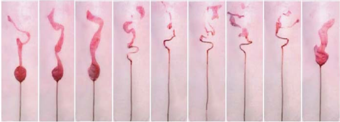
Figure 1.2. Bubble and spiral vortex breakdown Kurosaka et al. (2003).
