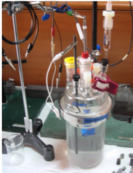
Figure 3.3: Electrochemical corrosion test system
