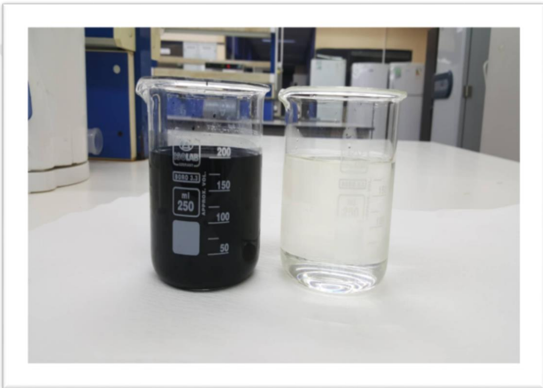
Figure 3.8: Decolorization of Black azo dyes by IE process.
