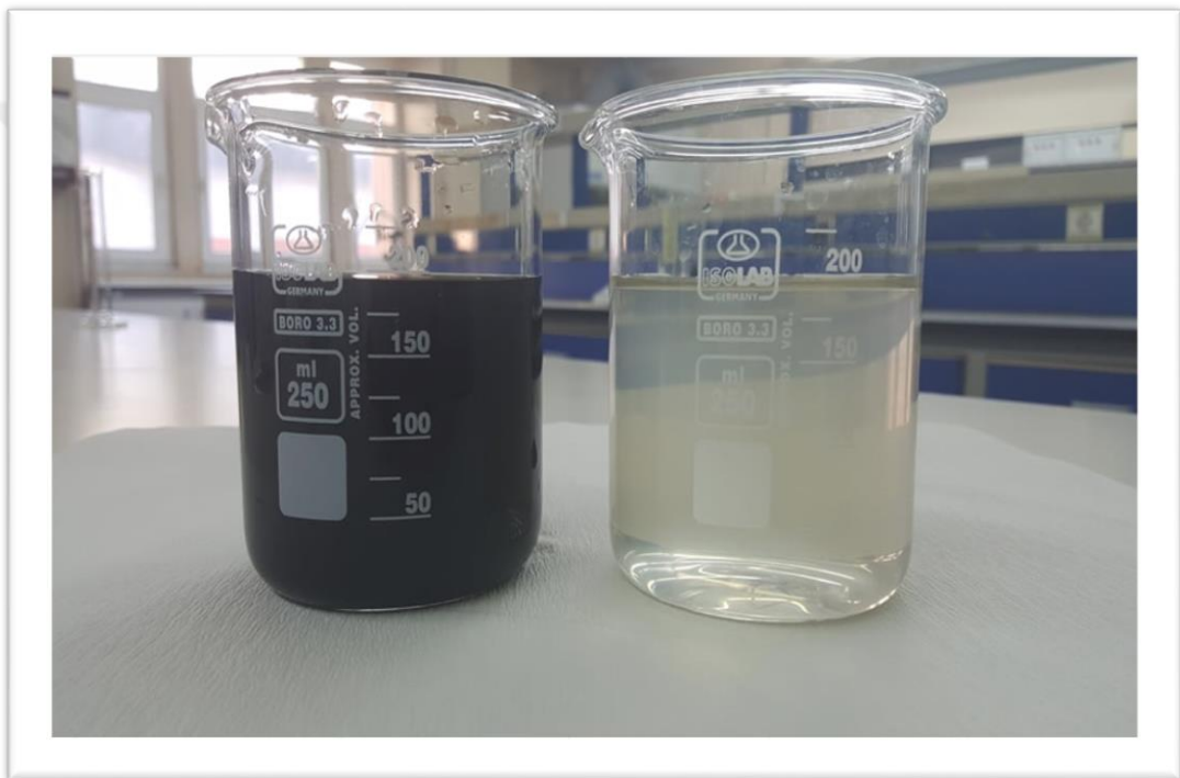
Figure 3.1: Decolorization of Raw textile wastewater by applying IE process.
