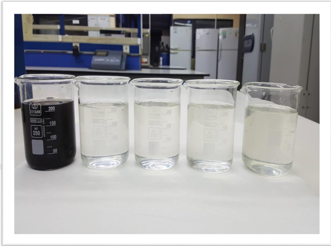
Figure 3.20: The performance of the 25 ml of anion resin ( \text{OH}^- ) used after regeneration (8 regeneration) with Chlorine and <5\% NaOH at ( 40^\circ\text{C} ).
