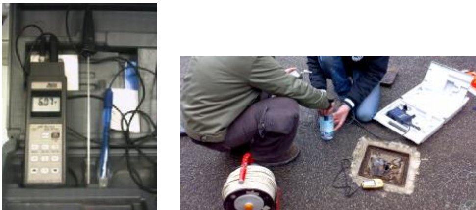
Figure 3.6. Measurement from a piezometer in Science Geology Department
