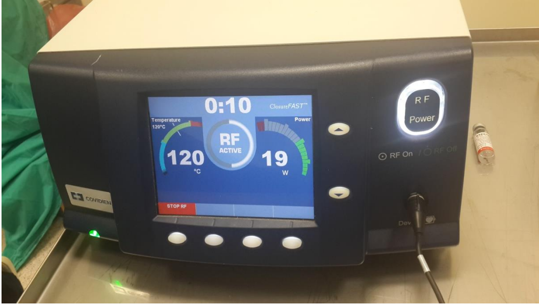
Resim 6. Bipolar Covidien ClosureRFG™ Radiofrequency Generator radyofrekans enerji kontrol ünitesi
