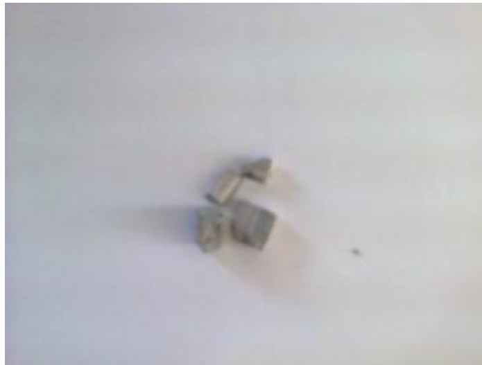
Figure 3.2. The cracked samples for measuring thermoelectric properties
