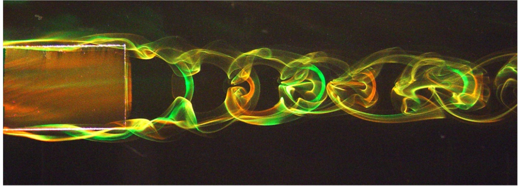
Figure 3.18. Dye visualization of the wake of an oscillating fin (IHHR,2015).
