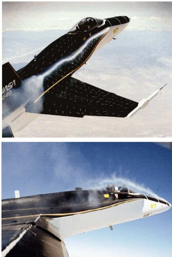
Figure 1.6. Vortex breakdown over NASA's F-18 aircraft at angle of attack \alpha=20^\circ and 42^\circ (Görtz, 2005).
