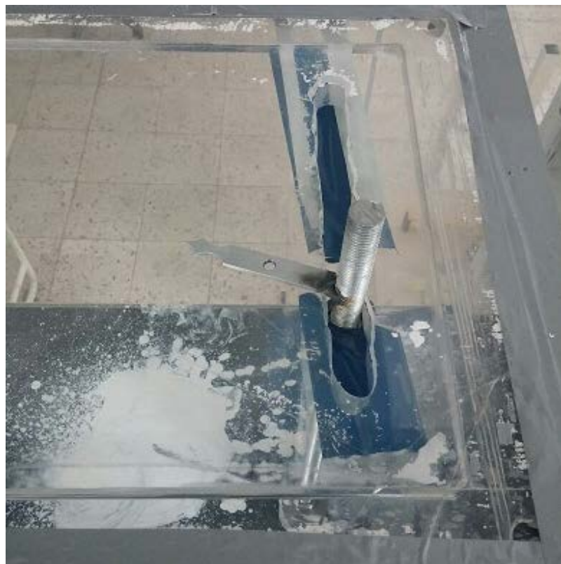
Figure 3.30. Channel on wind tunnel to move the delta wing to protect from wind tunnel wall's interference.
