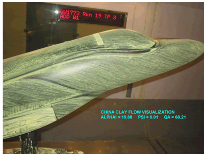
Figure 3.17. Oil visualization with China clay (UWAL, 2015).
