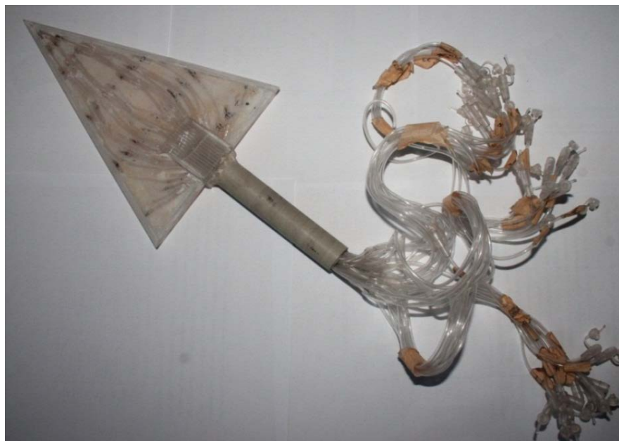
Figure 3.25. The delta wing used for pressure measurement.
