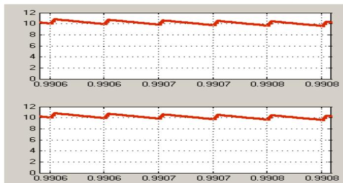
**Figure 5.60:** The inductors current at  $M=1.1$ ,  $V_{in}=198$  v.
