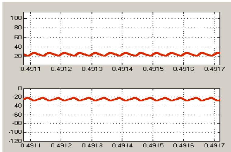
**Figure 5.22:** The Inductors current at  $M=0.755$ ,  $V_{in}=98$  v
