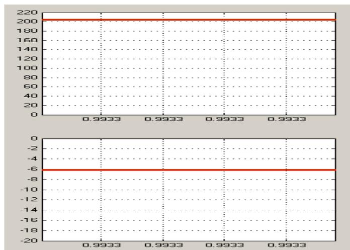
**Figure 5.59:** The voltage across  $C_1$  and  $C_2$  at  $M=1.1$ ,  $V_{in}=198$  v.
