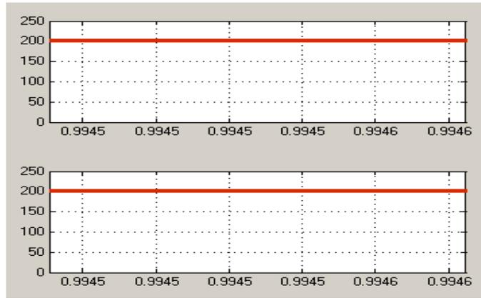
**Figure 5.42:** The voltage across  $C_1$  and  $C_2$  at  $M=1.1$ ,  $V_{in}=198$  v.
