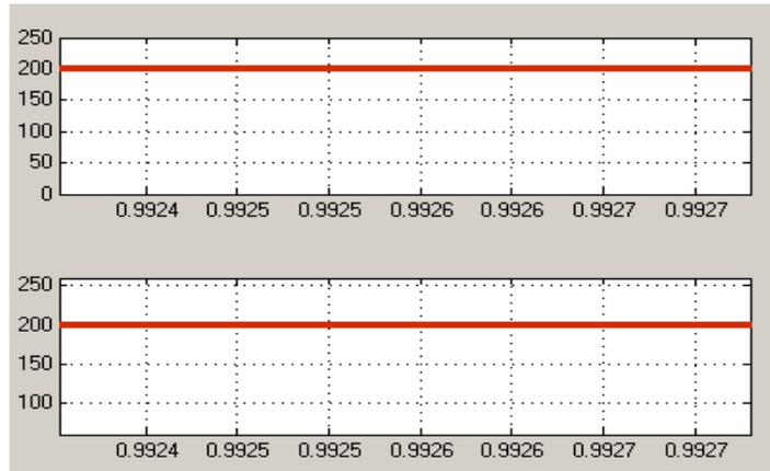
**Figure 5.34:** The voltage across  $C_1$  and  $C_2$  at  $M=1.0$ ,  $V_{in}=176$  v.
