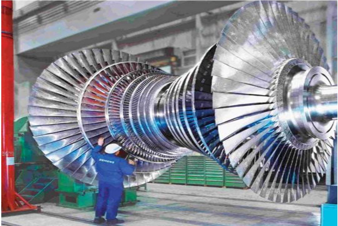
Figure 2.1: The rotor of a modern double-flow low-pressure steam turbine.
